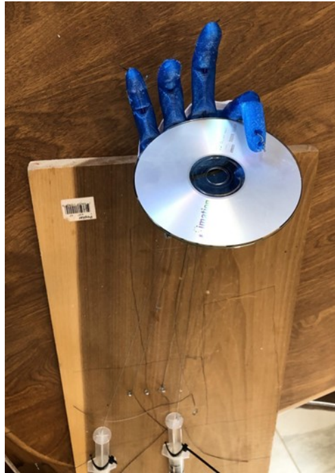
Figure 5 demonstrates the Ada Robot hand performing the pinch grip test. It also shows the Ada hand with the full hydraulic setup.
