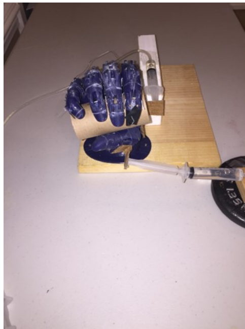
Figure 4 shows the unfinished robot hand performing the cylindrical test as proposed by Konnaris et al. (n.d.). The hand also has the full hydraulic setup attached.
