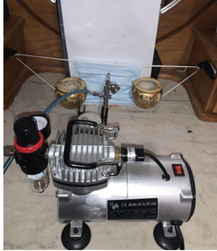
Figure 1 shows the experimental setup. The metal machine is the air compressor used for the airbrush. The hooks are located on the left and right side of the image. The airbrush is located in front of the mask. The two containers in the middle of the image are the 8-ounce weights used to hold the mask down. The paper is located on the clipboard.
