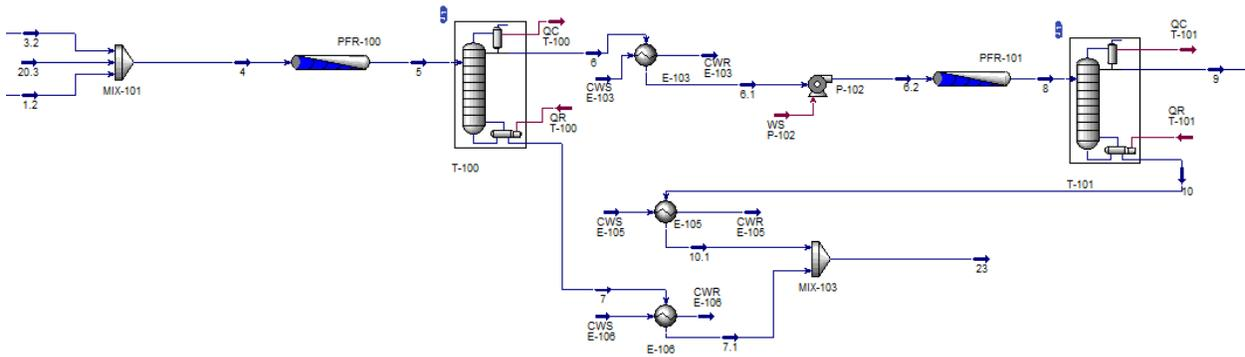
Figure 1: The process flow diagram of the base case generated in Aspen HYSYS.
