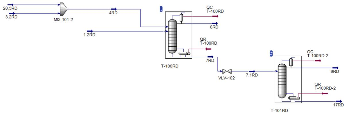
Figure 2: The process flow diagram of the reactive distillation case generated in Aspen HYSYS.
