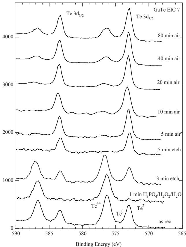
FIG. 2. XPS Te  $3d$  spectra for  $\text{H}_3\text{PO}_4:\text{H}_2\text{O}_2:\text{H}_2\text{O}$  etched and oxidized GaTe.
