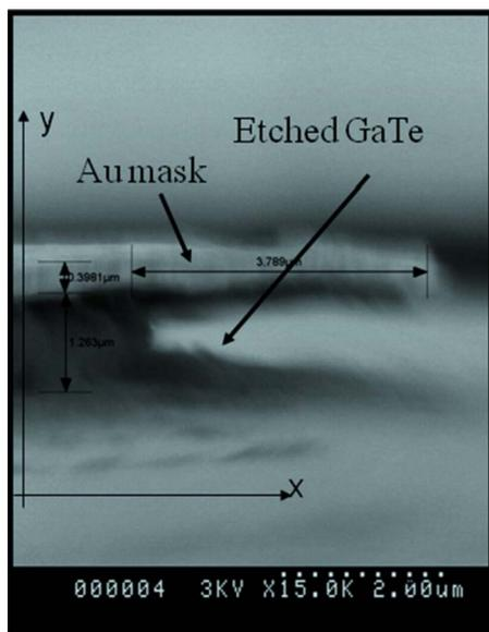
FIG. 9. (Color online) SEM picture of H<sub>3</sub>PO<sub>4</sub>:H<sub>2</sub>O<sub>2</sub>:H<sub>2</sub>O (1:1:10) etched GaTe.
