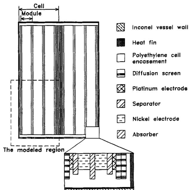
Fig. 4. Schematic representation of the nickel-hydrogen cell.
