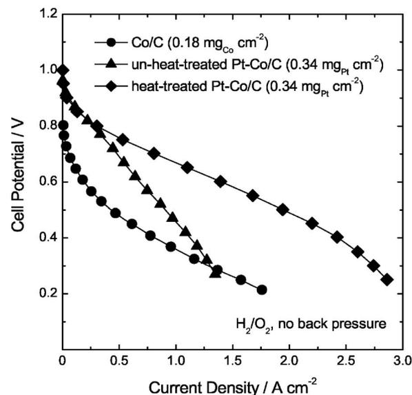
**Figure 3.** Polarization curves of the PEM fuel cells prepared with (i) Co/C, (ii) unheat-treated Pt-Co/C, and (iii) heat-treated Pt-Co/C. The experiments were performed under the following conditions: (i) Pt loading on the anode =  $0.5 \text{ mg cm}^{-2}$ , (ii)  $\text{H}_2$  flow rate =  $150 \text{ cm}^3 \text{ min}^{-1}$ , (iii)  $\text{O}_2$  flow rate =  $150 \text{ cm}^3 \text{ min}^{-1}$ , and (iv) cell temperature =  $75^\circ\text{C}$ .
