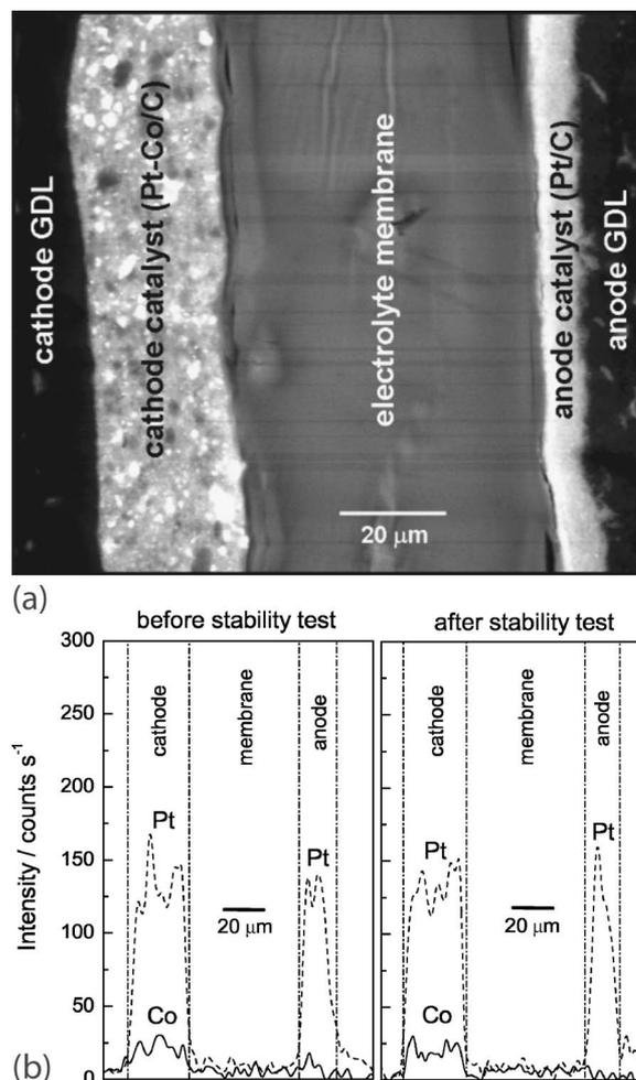
**Figure 6.** (a) BSEM images obtained from the cross sections of the fresh MEA with the Pt-Co/C catalyst developed in this study, and (b) concentration profiles of Pt and Co across the fresh MEA and the MEA subjected to 400 h of stability testing, obtained by EPMA cross section line scan.
