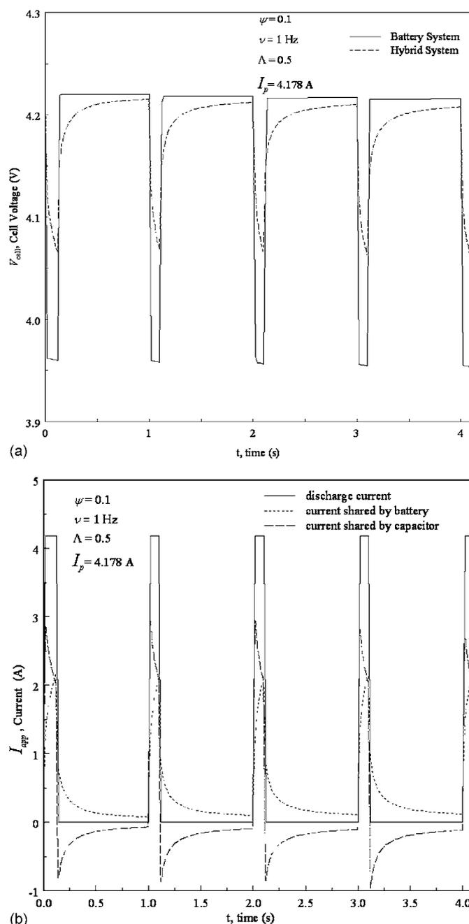
**Figure 2.** (a) Comparison of cell voltages for the battery and the hybrid system for short times. (b) Current shared by the battery and the capacitor for short times. Simulation results are for the case where  $\psi = 0.1$  and  $\nu = 1$  Hz.
