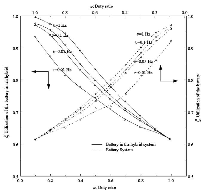
**Figure 7.** Plot showing the effect of duty ratio ( $\psi$ ) on the utilization ( $\xi$ ) of the pure battery and the battery in the hybrid system for various values of frequencies. The simulations are done for a current amplitude of  $I_p = 4.178$  A.
