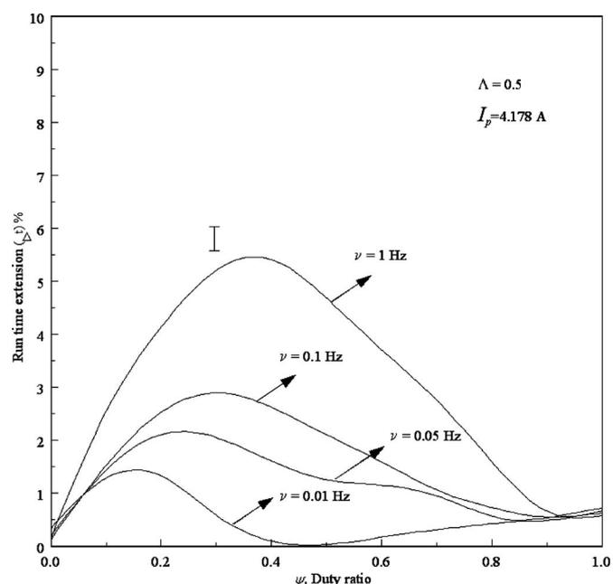
**Figure 8.** Simulated values of the percentage increase in the run time of the hybrid system over that of the battery system for different values of duty ratio. The effect of frequency on the run time extension of the hybrid system is also shown. The simulations are done for a current amplitude of  $I_p = 4.178$  A and discharged to 2.5 V.
