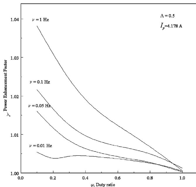
**Figure 9.** Power enhancement factor as a function of duty ratio. The effect of frequency on the power enhancement factor was also simulated. All simulations were done at  $I_p = 4.178$  A and capacitor configuration index  $\Lambda = 0.5$ .
