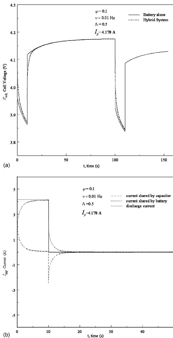
**Figure 4.** (a) Comparison of cell voltages for the battery and the hybrid system for short times. (b) Current shared by the battery and the capacitor for short times. Simulation results are for the case where  $\psi = 0.1$  and  $\nu = 0.01$  Hz.
