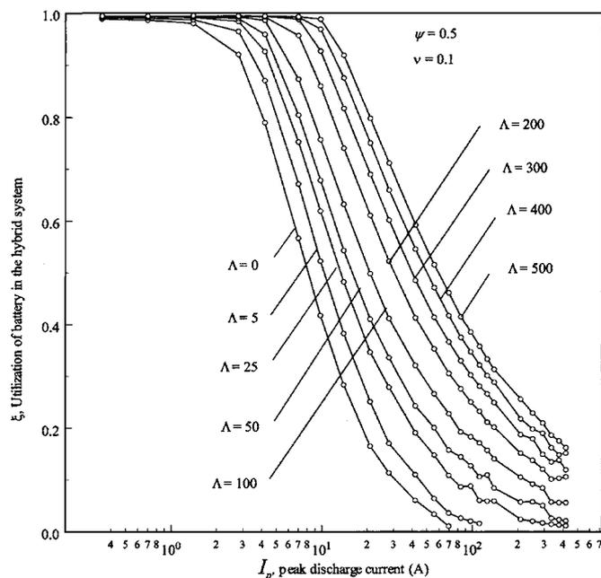
**Figure 10.** Simulated utilization of the battery as a function of discharge rate (peak pulse discharge current density). The plot also shows the better rate capability (high utilization at higher rates) at higher values of capacitor configuration index.
