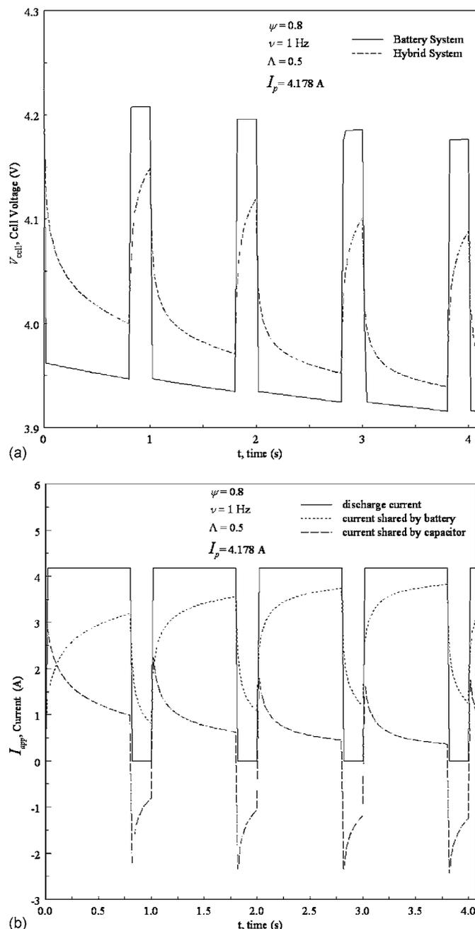
**Figure 3.** (a) Comparison of cell voltages for the battery and the hybrid system for short times. (b) Current shared by the battery and the capacitor for short times. Simulation results are for the case where  $\psi = 0.8$  and  $\nu = 1$  Hz.
