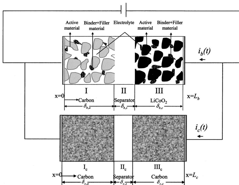
**Figure 1.** Schematic of a lithium-ion battery/electrochemical capacitor network hybrid system. The battery consisted of a positive  $\text{LiCoO}_2$  and negative carbon electrode with a separator while the electrochemical capacitor has carbon electrodes as anode and cathode sandwiched against a separator.
