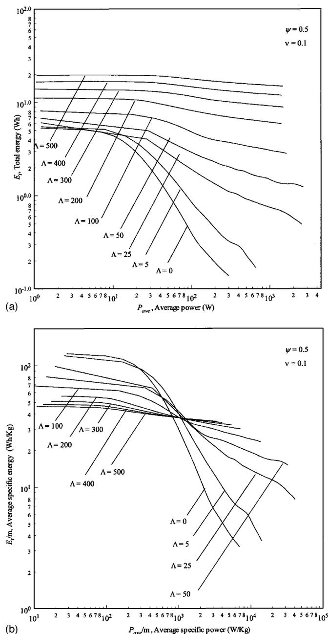
**Figure 11.** (a) Plot showing the total energy ( $E_t$ ) vs average power relationship for various values of capacitor configuration index,  $\Lambda$ . Each point on the curve was obtained by running the hybrid model at different pulse discharge rates. (b) Ragone plot comparison for the battery and hybrid system for various values of capacitor configuration index. This figure shows the improvement in the energy-delivering capacity of the hybrid system under high-power operations.
