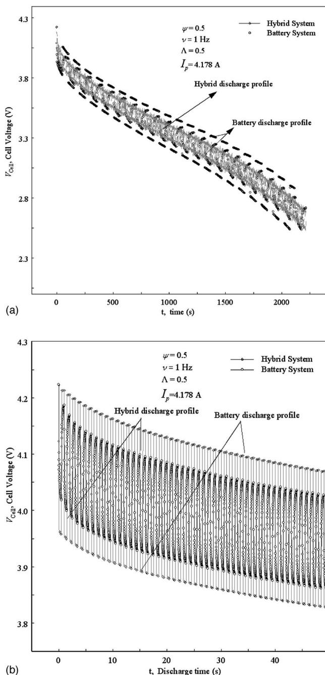
**Figure 6.** (a) Discharge curve for the pure battery system and hybrid system which shows the reduced voltage drop and the increased run time for the hybrid system as compared to the battery system. (b) Discharge curve for the pure battery system and hybrid system at short times. Simulated results are for the case  $\psi = 0.5$  and  $\nu = 1$  Hz.
