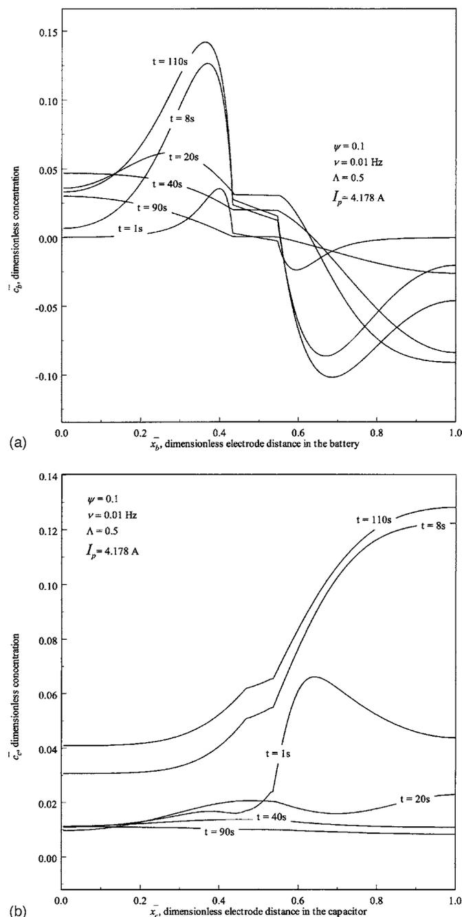
**Figure 5.** (a) Plot showing the concentration relaxation phenomenon in the (a) battery and (b) electrochemical capacitor during pulse discharge. Lines correspond to the dimensionless concentration profiles during the on time/off time of the pulse with the time marked on the curves.
