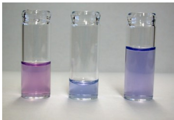
Figure 6: Liposomes prepared from 95% PCDA and 5% phenylalanine derivatized PCDA. 1) Treated with Salmonella; 2) Untreated 3) Treated with E. coli .
