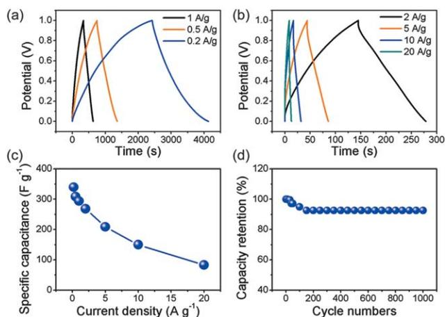
**Fig. 5** Constant current charge/discharge curves of the  $\beta$ -MnO<sub>2</sub>/polypyrrole nanorod composite electrode at different rates: (a) 0.2, 0.5, and 1 A g<sup>-1</sup>; (b) 2, 5, 10, and 20 A g<sup>-1</sup>. (c) Plot of specific capacitance as a function of current density. (d) Corresponding charge–discharge cycle.
