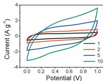
**Fig. 4** (a) Cyclic voltammograms of the MnO<sub>2</sub>/polypyrrole nanorod composite electrode in 1 M Na<sub>2</sub>SO<sub>4</sub> at the scan rates of 1, 2, 5, and 10 mV s<sup>-1</sup>, respectively.
