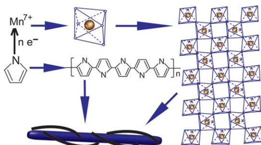
**Fig. 3** Schematic of the formation process of the β-MnO<sub>2</sub>/polypyrrole nanorod composite.
