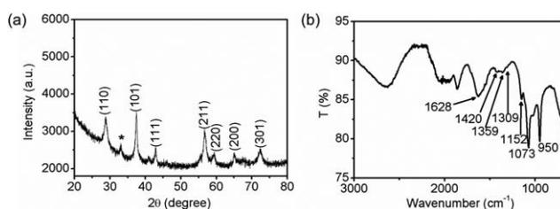
**Fig. 1** (a) XRD and (b) FTIR spectra of MnO<sub>2</sub>/polypyrrole nanorod composite powders.
