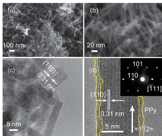
**Fig. 2** (a and b) Low- and high-magnification FESEM images of the  $\beta$ -MnO<sub>2</sub>/polypyrrole nanorod composite. (c and d) HRTEM analysis. The inset of panel (d) is its corresponding SAED pattern.
