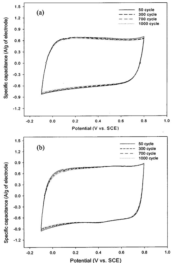
**Figure 11.** Cycle life tests of (a) Mn/PbO<sub>x</sub> and (b) Mn/NiO<sub>x</sub> in 1 M Na<sub>2</sub>SO<sub>4</sub> solution. Potential range between -0.1 and 0.8 V vs. SCE and scan rate 5 mV/s. The ratio of Mn/X is 8:2.
