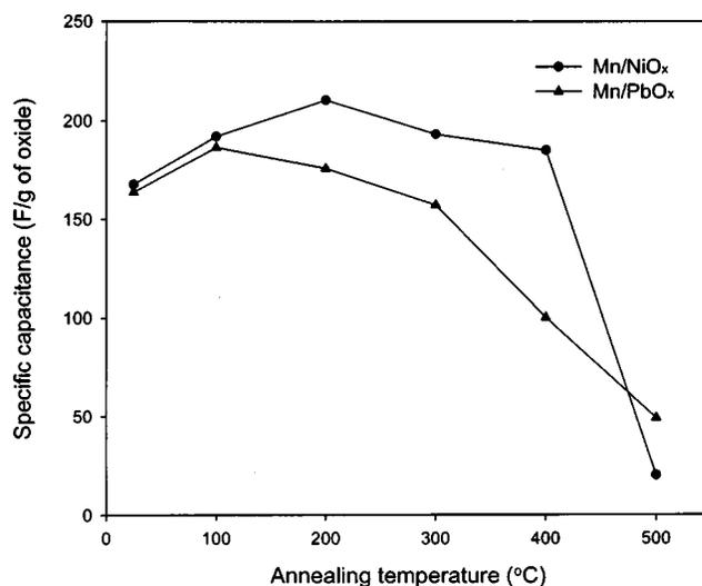
**Figure 2.** Effect of annealing temperature on the specific capacitance of Mn/PbO<sub>x</sub> and Mn/NiO<sub>x</sub>.
