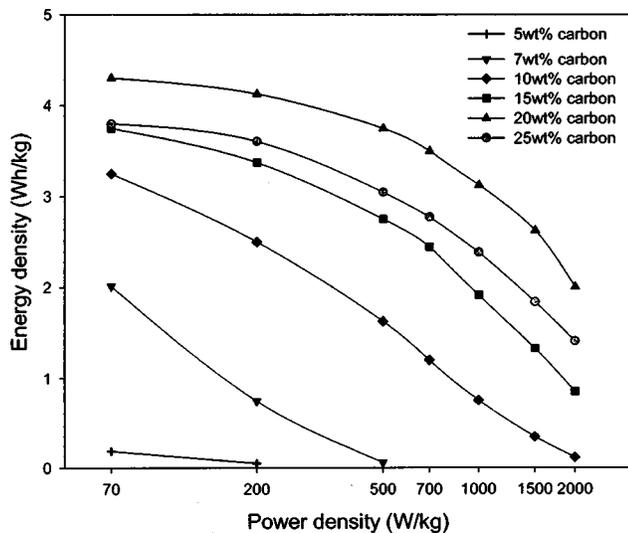
**Figure 9.** Ragone plot obtained for Mn/NiO<sub>x</sub> electrodes as a function of carbon loading. The ratio of Mn/Ni is 8:2.
