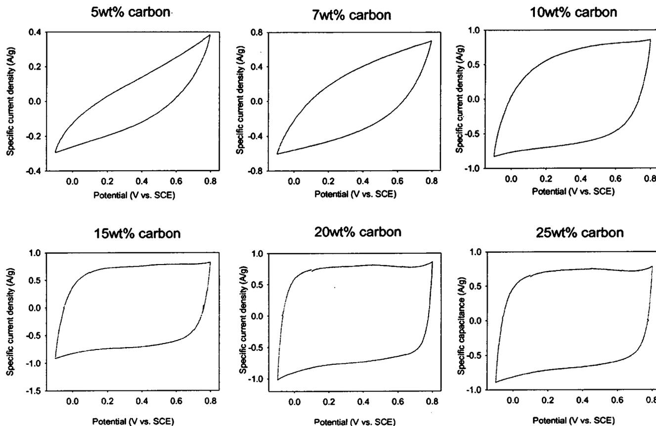
**Figure 8.** CVs of Mn/NiO<sub>x</sub> as a function of carbon content in the electrode in 1 M Na<sub>2</sub>SO<sub>4</sub> solution; potential range between -0.1 and 0.8 V vs. SCE and scan rate 5 mV. The ratio of Mn/Ni is 8:2.
