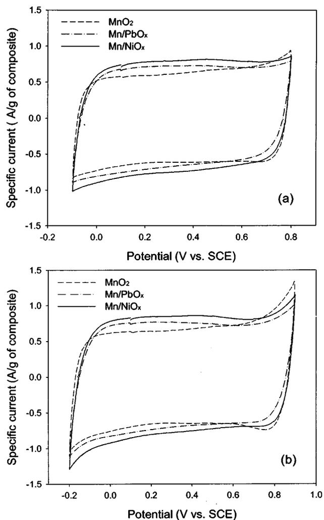
**Figure 1.** Cyclic voltammograms of MnO<sub>2</sub>, Mn/PbO<sub>x</sub>, and Mn/NiO<sub>x</sub> obtained at a scan rate of 5 mV/s in 1 M Na<sub>2</sub>SO<sub>4</sub>: (a) potential range between -0.1 and 0.8 V vs. SCE and (b) potential range between -0.2 and 0.9 V vs. SCE.
