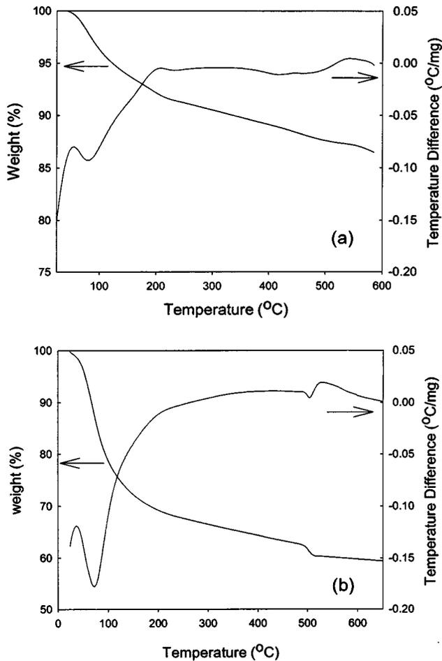
**Figure 5.** TGA and DTA of Mn/PbO<sub>x</sub> and (b) Mn/NiO<sub>x</sub> in He gas at 10°C/min. The ratio of Mn/X is 8:2.
