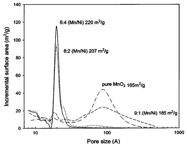
**Figure 7.** BET surface area and pore size distribution of Mn/NiO<sub>x</sub> for different Ni loadings.
