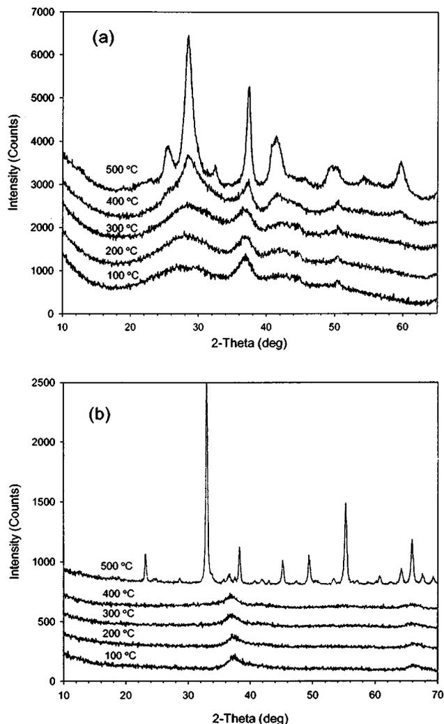
**Figure 3.** XRD patterns of (a) Mn/PbO<sub>x</sub> and (b) Mn/NiO<sub>x</sub> as a function of annealing temperature. The ratio of Mn/X is 8:2.
