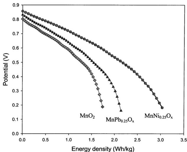
**Figure 10.** Discharged energy density curves of MnO<sub>2</sub>, Mn/Pb, and Mn/Ni mixed oxides obtained at the constant power discharge of 1 kW/kg. The ratio of Mn/X is 8:2 and carbon ratio is 20 wt %.
