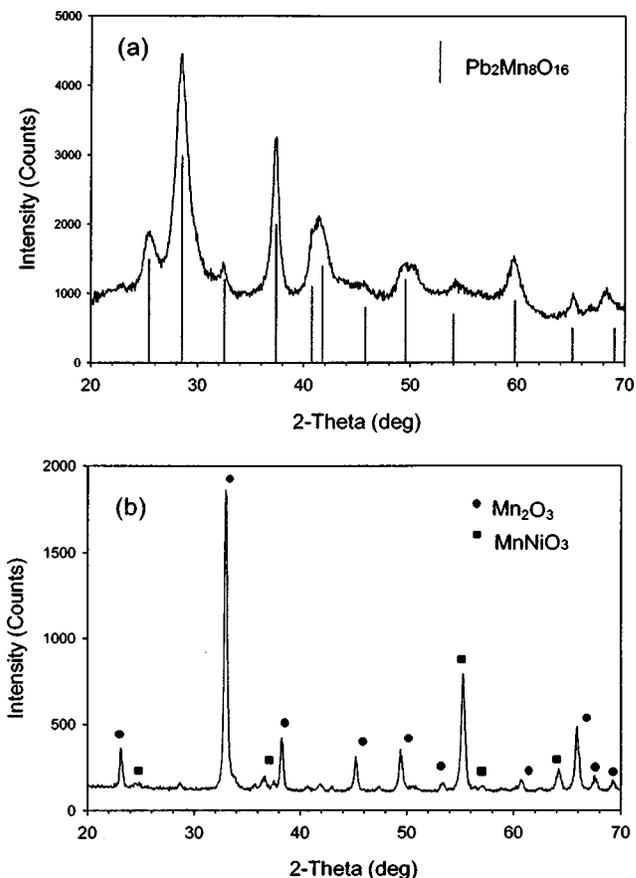
**Figure 4.** XRD patterns of (a) Mn/PbO<sub>x</sub> and (b) Mn/NiO<sub>x</sub> annealed at 500°C.
