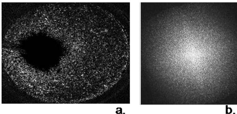
Figure 2. a.) Fluctuation image determined by subtracting two normalized frames at a time delay of  $\Delta t = 100$  s. The large dark area is the subtracted region where the light source is fed into the system underneath the sample cell. This figure gives a top down view into the sample cell. b.) Corresponding power spectrum after performing a 2D FFT on the fluctuation image.
