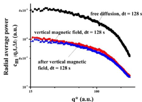
Figure 5. Power spectrum comparison at a delay time of 128 s. Nanoparticles that have been exposed to a magnetic field, even if not currently exposed to a magnetic field, still exhibit a smaller amplitude of the power spectrum than that of free diffusion.
