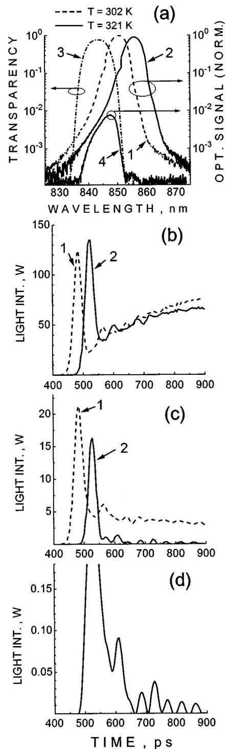
FIG. 3. Time-integrated lasing spectra (a), nonfiltered (b) and filtered (c) optical pulse waveforms. The curves 1 were measured at a laser diode temperature of  $302^{\circ}\text{K}$ , and the curves 2 at  $321^{\circ}\text{K}$ . Curve 3 in (a) shows the spectral characteristics of the filter, and curve 4 presents the filtered spectrum at  $321^{\circ}\text{K}$  corresponding to the single pulse. The bottom of the single pulse [curve 2 in (b)] is shown at a higher amplification in (d).
