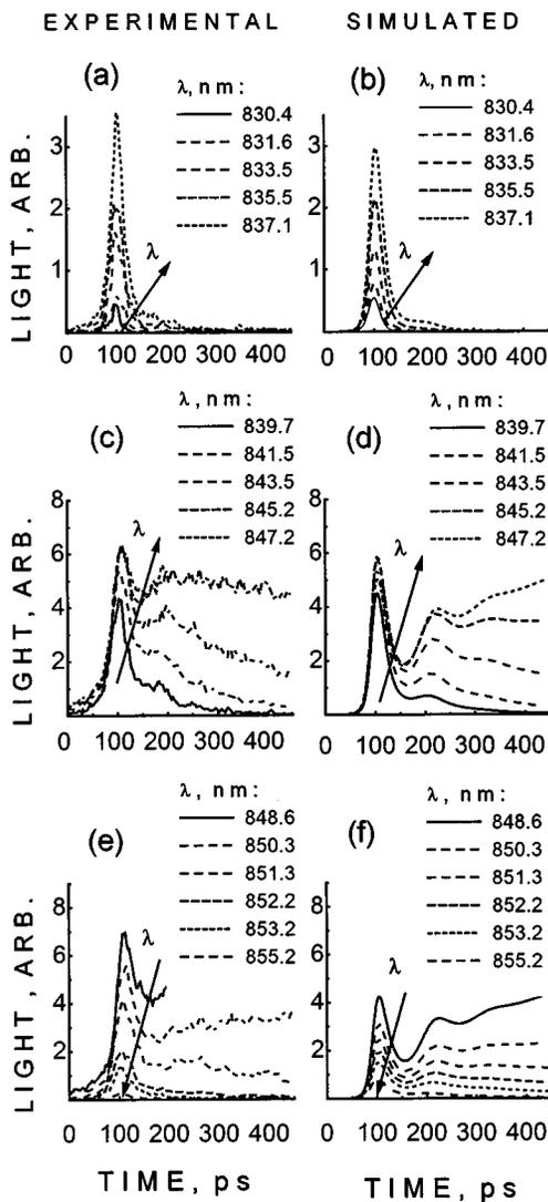
FIG. 2. Experimental and simulated monochromatic traces from the response of the gain-switched laser diode. Diode temperature  $T=292^{\circ}\text{K}$ . Modes 17, 18 (wavelengths 857.2 and 859.2 nm, respectively) are omitted because their intensities are negligible.
