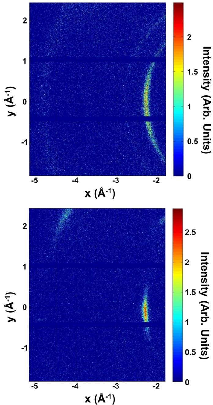
Figure 2: 2D area diffraction patterns from an as-deposited top) polycrystalline ScSZ sample deposited at 500°C and no O<sub>2</sub> and a bottom) textured ScSZ deposited at 500°C and 5 vol.% O<sub>2</sub>.
