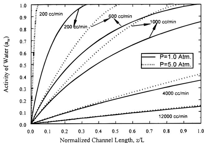
**Figure 6.** Simulated water activity vs. normalized channel length for 1.0 and 5.0 atm cell pressure and 80°C. The dashed curves represent simulations for 5.0 atm and the solid curves represent then 1.0 atm case. The activity of water decreases with an increase in the flow rate of nitrogen. When the activity of water reaches unity, water condenses in the flow channel.
