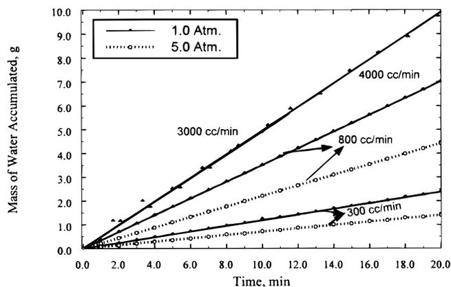
**Figure 3.** Plot of mass of water accumulated in the knock-out vessel vs. time. Symbols represent experimental data, and the lines indicate regressed linear fits. The slopes of the regressed fits were used to calculate the flux of water. The straight-line behavior is indicative of a steady-state process.
