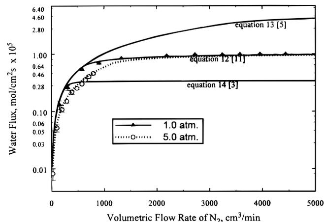
**Figure 4.** Simulated and experimental water flux data as a function of the volumetric flow rate of nitrogen at 80°C. The symbols represent experimental data, and the curves represent model simulations. Use of Eq. 12 for the Fickian diffusion coefficient of water results in an accurate prediction of the flux of water across the membrane. Calculations based using Eq. 13 and 14 over and under predict the flux of water, respectively.
