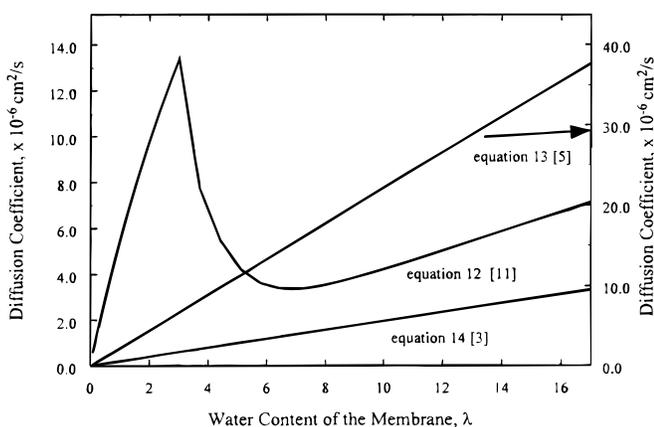
**Figure 2.** Fickian diffusion coefficient values reported by Fuller (Eq. 13),<sup>5</sup> Nguyen and White (Eq. 14),<sup>3</sup> and Zawodzinski *et al.* (Eq. 12)<sup>11</sup> at a temperature of 80°C. Equations 13 and 14 are linearly dependent on the water content of the membrane. Equation 12 shows a maximum at  $\lambda = 3$  due to the nature of the equilibrium relationship as given by 7.
