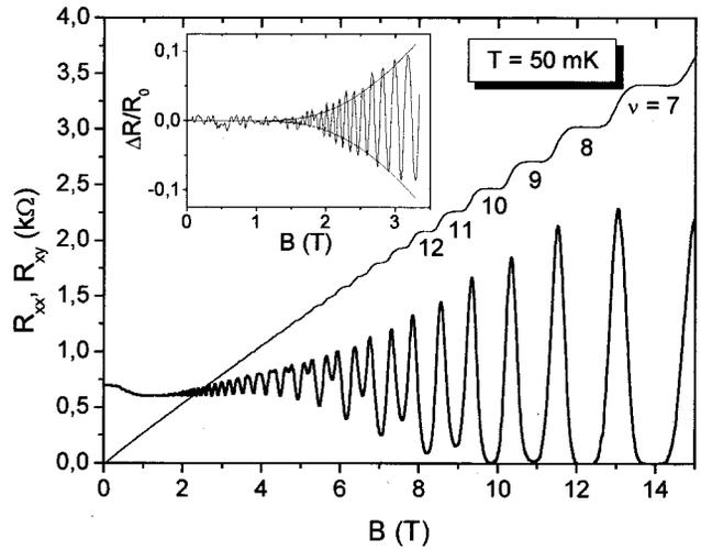
FIG. 2. Longitudinal ( $R_{xx}$ ) and transverse ( $R_{xy}$ ) magnetoresistance vs magnetic field at 50 mK. Shubnikov de Hass oscillations begin at 1.8 T. The inset shows  $\Delta R/R_0 = (R_{xx} - R_0)/R_0$ —the low-field part of  $R_{xx}$  after normalization by the zero-field resistance value  $R_0$ . The best fit of the SdHOs amplitude yields the value of  $T_D = 3$  K.
