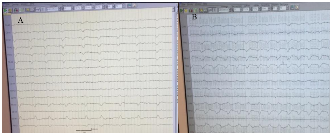
Figure 11. EEG electrode signals of the subject blinking slowly comparing the conductive plastic cups coated in Ag/AgCl to the control. Each dip in the signal represents a blink. (A) Conductive plastic cups coated in Ag/AgCl. (B) Control.
