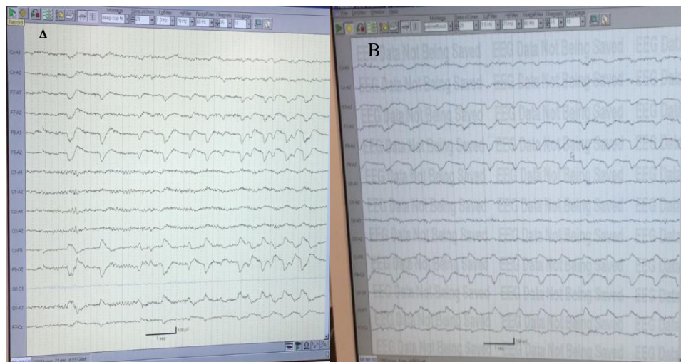
Figure 9. EEG electrode signals of the subject blinking slowly for the two control trials. Each dip in the signal represents a blink. Size and frequency of the dips may change due to the duration and speed of the blinks. (A) Control A. (B) Control B.
