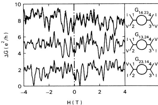
FIG. 1. Magnetoconductance  $\Delta G$  measured at  $T=0.04$  K for lead configurations 1423 [ $I(1 \rightarrow 4)$  and  $V(2 \rightarrow 3)$ ], 1324, and 2314 as marked. The dashed line is a different trace for configuration 1423 which indicates the reproducibility in the measurement. The Aharonov-Bohm oscillations ( $h/e$  and  $h/2e$ ) have been filtered from the data digitally.
