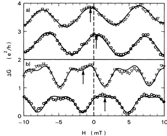
FIG. 3. (a) The asymmetry of the Aharonov-Bohm oscillations for the ring of Fig. 1 for  $G_{14,23}$  (circles) and  $G_{23,14}$  (inverted triangles). (b) The same measurement for a different ring of similar dimensions. The lines are fitted to the data and the arrows indicate the maximum of the cosine function for the fundamental frequency. These oscillations were studied in a low magnetic field environment.
