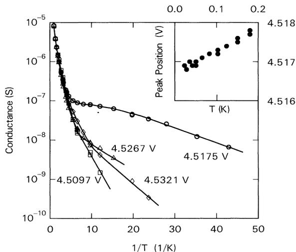
FIG. 2. Temperature dependence of four conductance peaks shown in Fig. 1 at  $V_G = 4.5097$ ,  $4.5175$ ,  $4.5267$ , and  $4.5321$  V with activation energies 36, 7.2, 13, and 18  $\mu$ eV, respectively. Solid lines are smooth curves through the data. The inset shows the temperature dependence of the peak position for the peak at  $V_G = 4.5175$  V in the temperature regime where the peak is isolated from its neighboring peaks.
