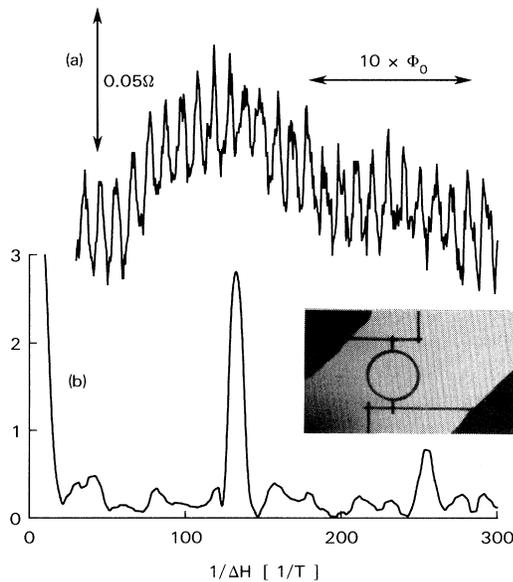
FIG. 1. (a) Magnetoresistance of the ring measured at  $T=0.01$  K. (b) Fourier power spectrum in arbitrary units containing peaks at  $h/e$  and  $h/2e$ . The inset is a photograph of the larger ring. The inside diameter of the loop is 784 nm, and the width of the wires is 41 nm.
