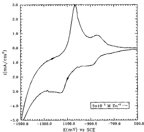
Fig. 2. The enlarged cyclic voltammetry curve presented in Fig. 1 for the concentration of 5 × 10<sup>-3</sup> M Zn<sup>+2</sup>.
