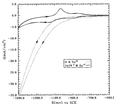
Fig. 1. Cyclic voltammetry curves obtained on Monel K500, using an electrolyte containing 1M Na<sub>2</sub>SO<sub>4</sub>, 0.4M NaCl, and 1M H<sub>3</sub>BO<sub>3</sub> in the absence and presence of Zn<sup>+2</sup>, and sweep rate = 100 mV/s.
