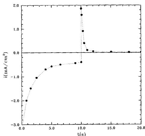
Fig. 5. A typical cathodic and anodic transient for Monel K500 in the electrolyte containing 1M  $\text{Na}_2\text{SO}_4$ , 0.4M NaCl, and 1M  $\text{H}_3\text{BO}_3$  in the presence of  $5 \times 10^{-3}$  M of  $\text{Zn}^{+2}$ ,  $t_c = 10$  s,  $E_c = -1.0$  V.
