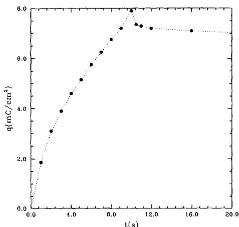
Fig. 6. A typical charge accumulation during the charge and discharge process for Monel K500 in an electrolyte containing 1M  $\text{Na}_2\text{SO}_4$ , 0.4M NaCl, and 1M  $\text{H}_3\text{BO}_3$  in the presence of  $5 \times 10^{-3}$  M  $\text{Zn}^{+2}$ ,  $t_c = 10$  s,  $E_c = -1.0$  V.
