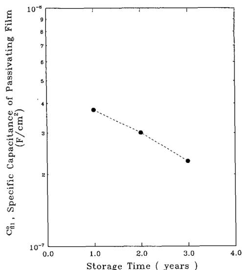
Fig. 8. Dependence of the specific capacitance of the LiCl passivating film,  $C_{fi}^0$  on battery storage time.
