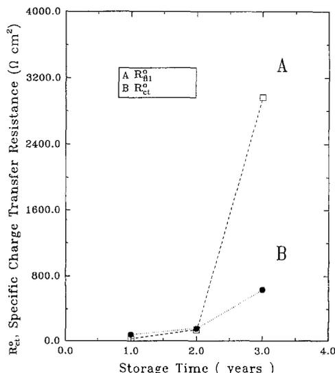
Fig. 12. Relationship between specific charge-transfer resistance and storage time. A, film/electrolyte,  $R_{12}^0$ ; B, Li anode/film,  $R_{ct}^0$ .
