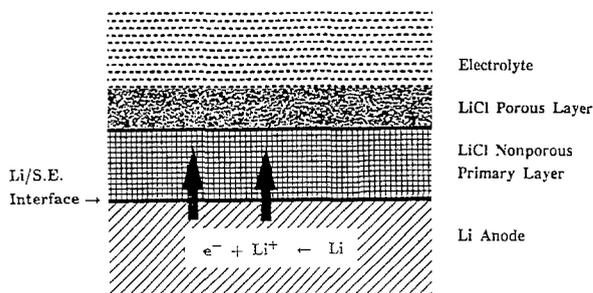
Fig. 1. Schematic representation of a passivated lithium anode in SOCl<sub>2</sub> solution at open circuit.
