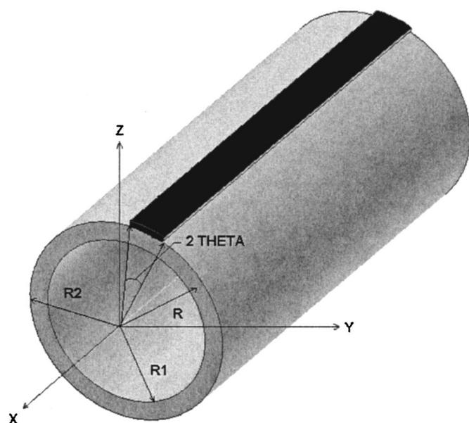
**Figure 1.** A geometrical schematic of O<sub>2</sub> pore diffusion under cylindrical coordinate system.
