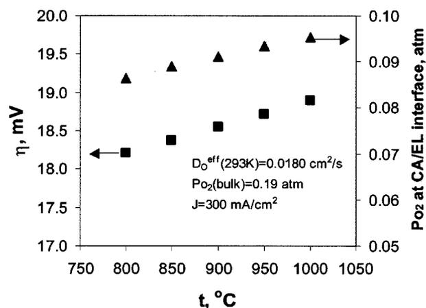
**Figure 2.** Pore polarization and interfacial  $p_{\text{O}_2}$  as a function temperature. CA/EL represents cathode/electrolyte.
