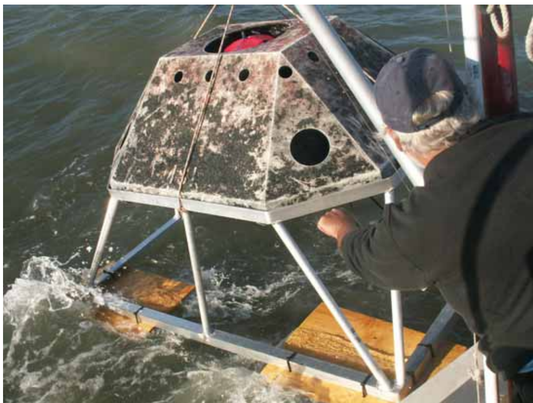
Fig. 7: Marine Research Division's Carl Naylor lowers the now-replaced ADCP unit in its trawl-proof shell to the muddy seafloor off Folly Pier. ( SCIAA photo )
