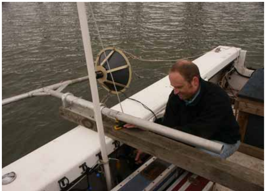
Fig. 3: Scott White, a researcher in USC's Department of Geological Sciences prepares a sub-bottom profiler for use aboard the Marine Research Division's C-Hawk . (SCIAA photo)
