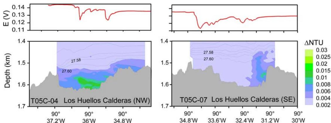
**Figure 6.** Hydrothermal plumes over the Los Huellos calderas on the east limb of the GSC. (top) Profiles of  $E$  from DSL-3. (bottom) Contoured  $\Delta NTU$  data from CTDOs through the calderas. The CTDO towpaths closely followed the DSL towpath. Potential density isopycnals are overlain.
