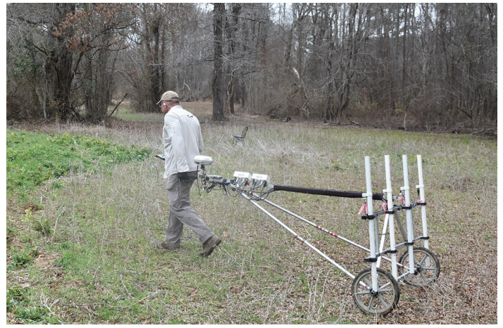
Figures 3a and 3b: (Left) Adamson Mound, (Right) Chet Walker conducting the survey with his Bartington Grad 601-4 fluxgate gradiometer. (Photos by Chris Judge)
