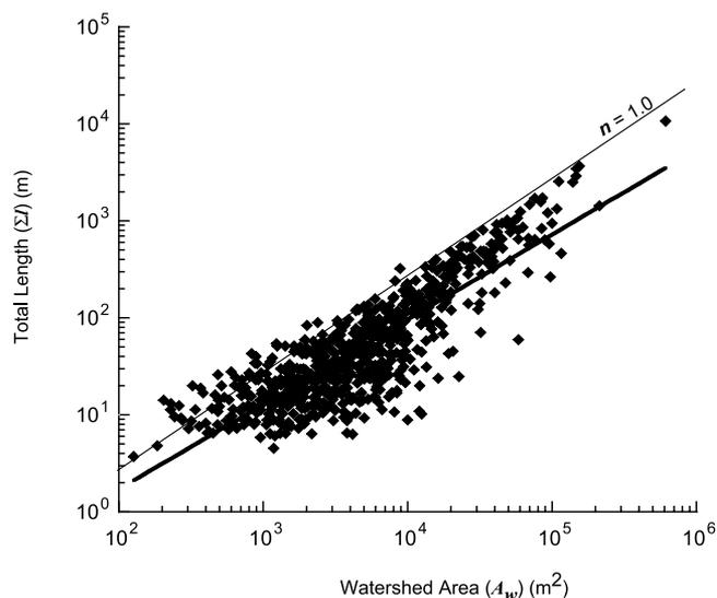
**Figure 10.** Total network length ( $\Sigma l$ ) versus watershed area ( $A_w$ ). Regression  $\Sigma l = 0.03A_w^{0.88}$ , shown as a thick solid line,  $r^2 = 0.85$ . Upper limit with a slope of 1.0 is shown as a thin solid line.
