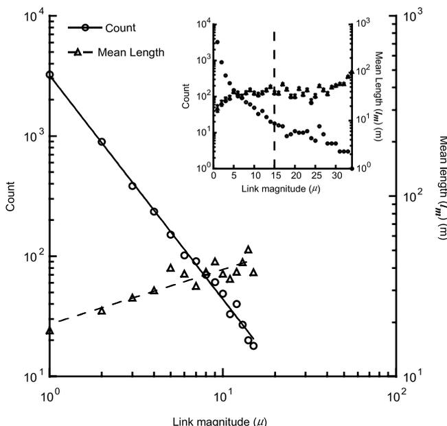
**Figure 5.** Magnitude ( $\mu$ ) versus number of creek segments and the mean length ( $l_m$ ) for  $\mu$  1–15. Inset shows relationship for  $\mu$  1–33. Vertical line indicates where scatter increases significantly. Standard errors on each mean value are represented by error bars.
