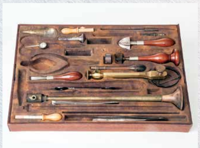
Tray of tools from Thomas Cooper's blowpipe kit used to identify minerals (photo by Matt Collins)
