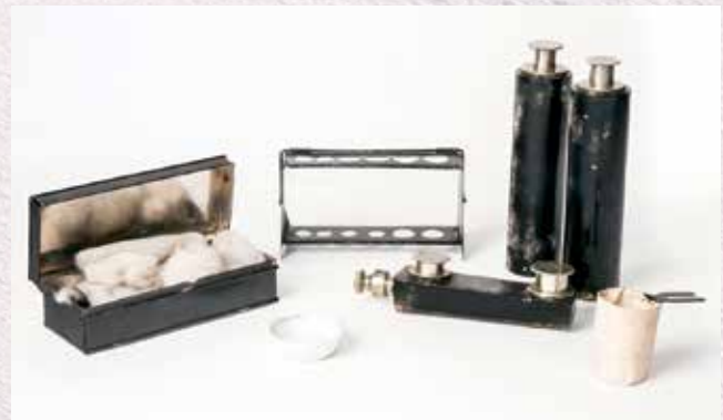
Fuel equipment used by Thomas Cooper to burn ground minerals for identification via blowpipe analysis (photo by Matt Collins)
