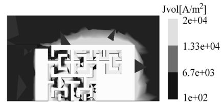
Fig. 6. Current distribution of antenna A at 2.45 GHz.
