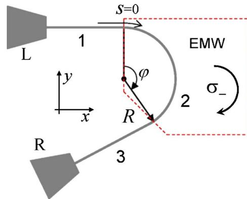
FIG. 1. (Color online) Curved quantum wire irradiated by a circularly polarized electromagnetic wave (EMW) with the electric field component precessing in  $x$ - $y$  plane. It is assumed in our model that the curved quantum wire consists of two straight segments 1 and 3 connected by an arc 2.
