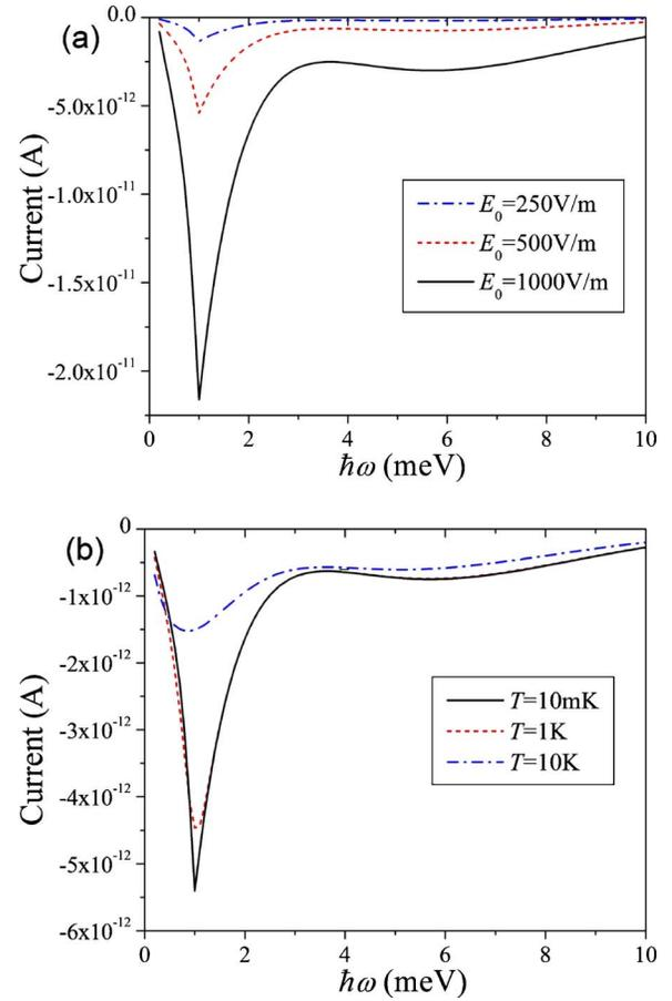
FIG. 3. (Color online) A photocurrent as a function of the photon energy calculated (a) for different radiation intensities at  $T=10$  mK and (b) for different temperatures at  $E_0=500$  V/m. The other parameters values are as in Fig. 2 with  $\varphi=\pi$  and  $R=25$  nm.
