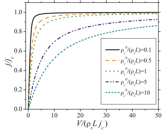
FIG. 2. (Color online) Current-voltage characteristics of the system calculated for several values of the ratio between the contact resistance and the semiconductor resistance  $\rho_c^0/(\rho_s L)$  (see text for details).
