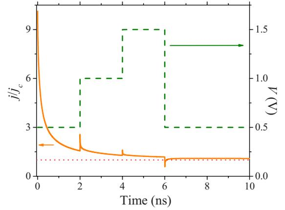
FIG. 5. (Color online) Transient current (solid line) excited by application of step voltages (dashed line). The dotted horizontal line, corresponding to  $j = j_c$ , is a guide for the eyes. Here we used  $L = 20 \mu\text{m}$  and  $\rho_c^0/(\rho_s L) = 1$ . The rest of the parameters are shown in Fig. 4.
