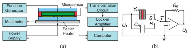
FIG. 2. (Color online) (a) Experimental setup. (b) A capacitance/voltage transformation circuit for sensor admittance measurements.
