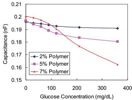
FIG. 5. (Color online) Equivalent capacitance of the microsensor with the polymer containing glucose monosaccharides galactose or fructose at varying concentrations (frequency: 100 kHz).
