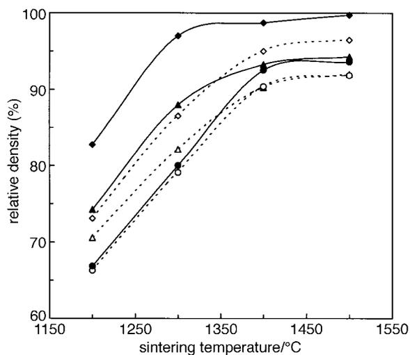
Fig. 8 Sintered density as a function of temperature at the following calcination temperatures: ( $\Delta$ ,  $\blacktriangle$ ) 1000, ( $\diamond$ ,  $\blacklozenge$ ) 1100, ( $\circ$ ,  $\bullet$ ) 1200 °C. Open symbols: samples of ground powders; filled symbols: samples of ball-milled powders.
