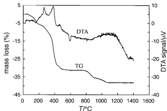
Fig. 3 DTA-TG curve for the oxalate coprecipitated powder
