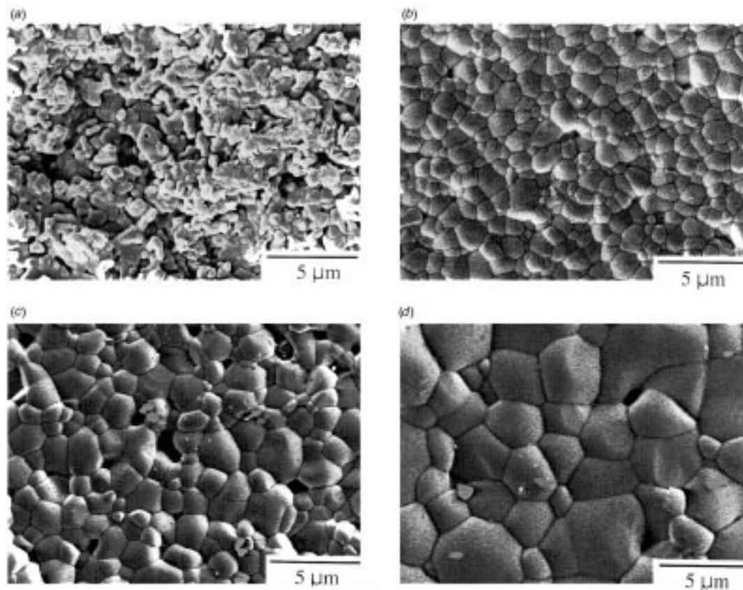
**Fig. 10** Scanning electron micrographs of sintered surface. Sintering temperature: (a) 1200 °C, (b) 1300 °C, (c) 1400 °C, (d) 1500 °C.
