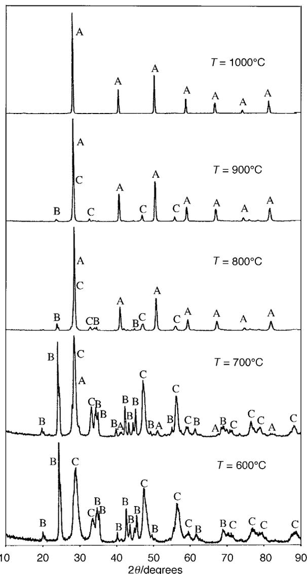
**Fig. 4** X-Ray diffraction patterns of the precipitate heated at the temperatures indicated for 8 h. A, B and C indicate diffraction peaks produced from  $\text{BaCe}_{0.9}\text{Nd}_{0.1}\text{O}_{3-\delta}$ ,  $\text{BaCO}_3$  and  $\text{CeO}_2$ , respectively.
