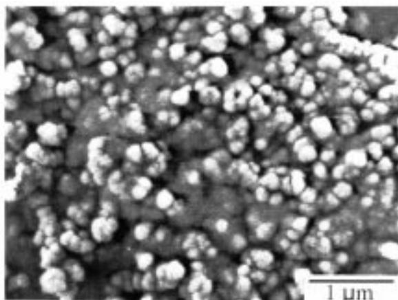
Fig. 2 Scanning electron micrograph of the precipitate powders
