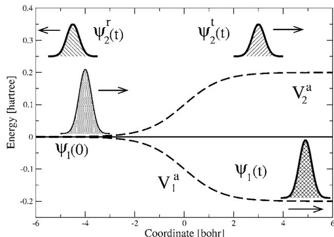
FIG. 3. Extended coupling with reflection. Adiabatic potential surfaces  $V_1^a$  and  $V_2^a$  are shown with dashed lines; diabatic potential surfaces shown with a single solid line have a small splitting of  $1.2 \times 10^{-3}$  hartree.
