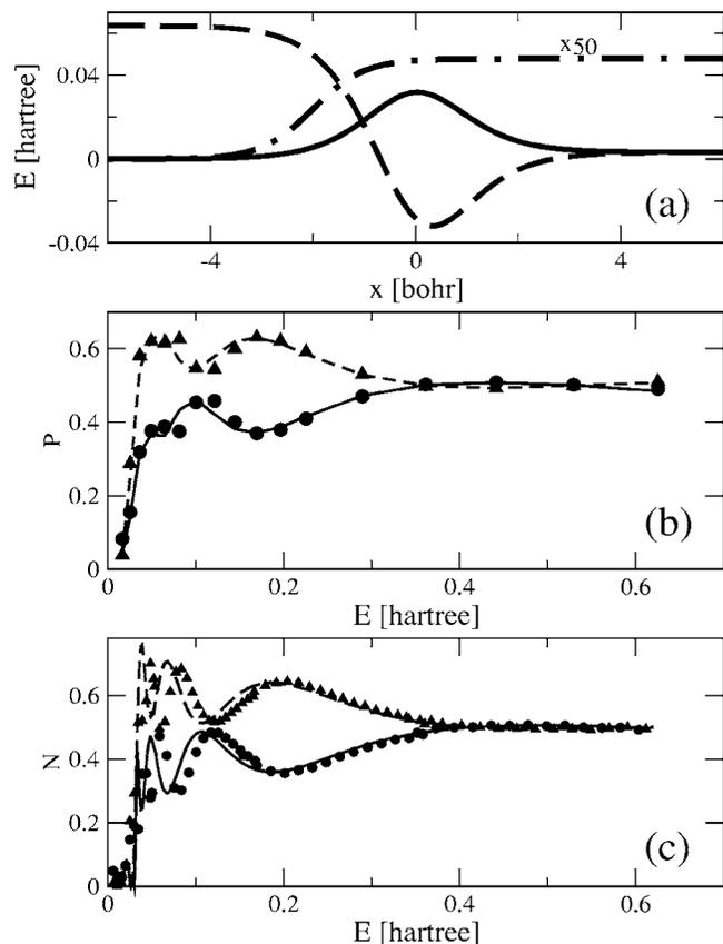
FIG. 2. Weak extended coupling. (a) Potential surfaces,  $V_1$  (solid line),  $V_2$  (dashed), and coupling  $V_{12}$  (dot-dashed). (b) The wave-packet probabilities as a function of the initial energy of the wave packet: quantum mechanical  $P_{11}$  and  $P_{12}$  are shown with solid line and dashed, respectively; semiclassical  $P_{11}$  and  $P_{12}$  are shown with circles and triangles, respectively. (c) The energy-resolved probabilities. Legend is the same as in (b).
