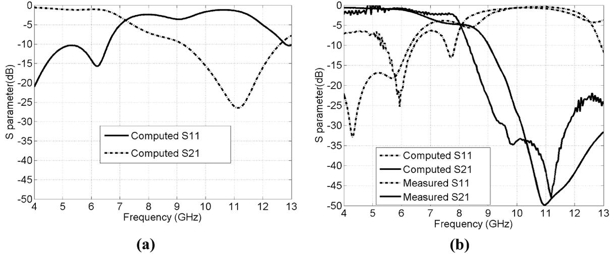
Fig. 4. S-parameters of (a) filter 1 and (b) filter 2.
