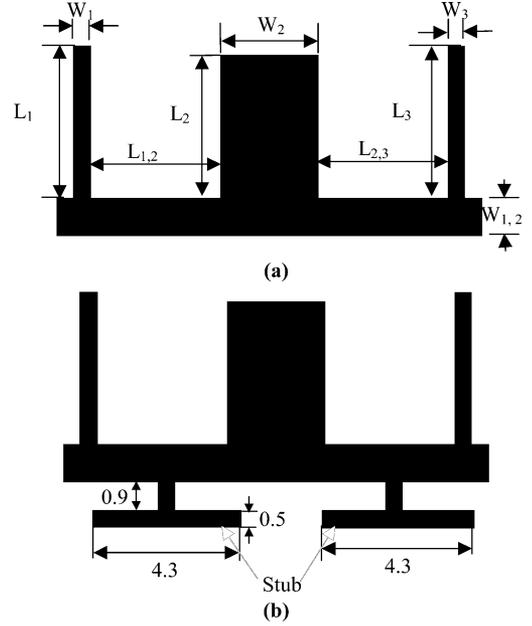
Fig. 3. Geometry of (a) band-reject filter 1 and (b) band-reject filter 2 (unit: mm).
