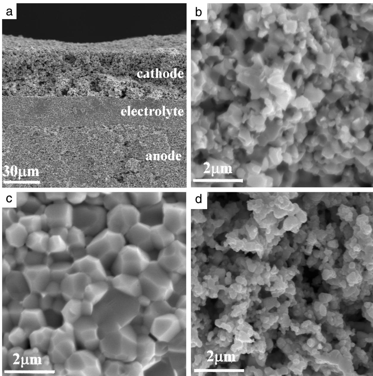
**Figure 1.** Cross-sectional view (SEM graphs) of (a) a single cell, (b) the porous Ni-SDC anode, (c) the dense SDC electrolyte, and (d) the porous  $\text{Sm}_{0.5}\text{Sr}_{0.5}\text{CoO}_3 + 10 \text{ wt } \% \text{ SDC}$  cathode.
