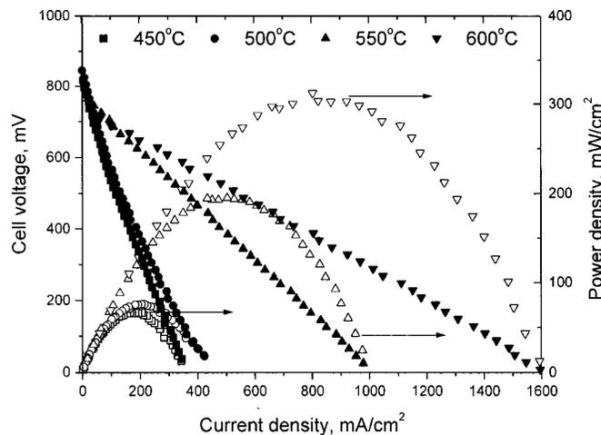
**Figure 4.** Cell voltages (solid symbols) and power densities (open symbols) as a function of current densities for an SOFC with humidified (3% H<sub>2</sub>O) methane as fuel at temperatures from 450 to 600°C.
