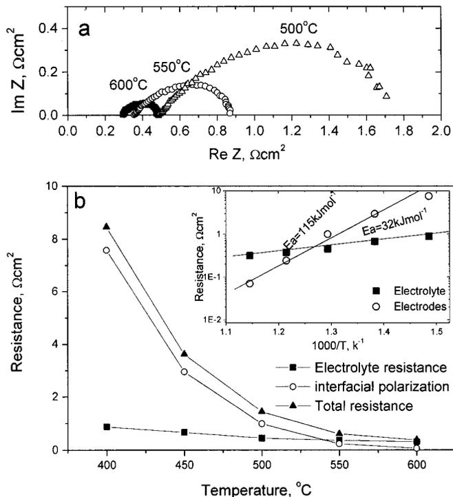
**Figure 3.** (a) Impedance spectra of an SOFC (Ni-SDC/SDC/Sm<sub>0.5</sub>Sr<sub>0.5</sub>CoO<sub>3</sub>) as measured under open-circuit conditions when humidified H<sub>2</sub> was used as fuel and air as oxidant at 500, 550, and 600°C. (b) Electrolyte resistance, interfacial polarization resistance, and total cell resistance as determined from the impedance spectra shown in (a).
