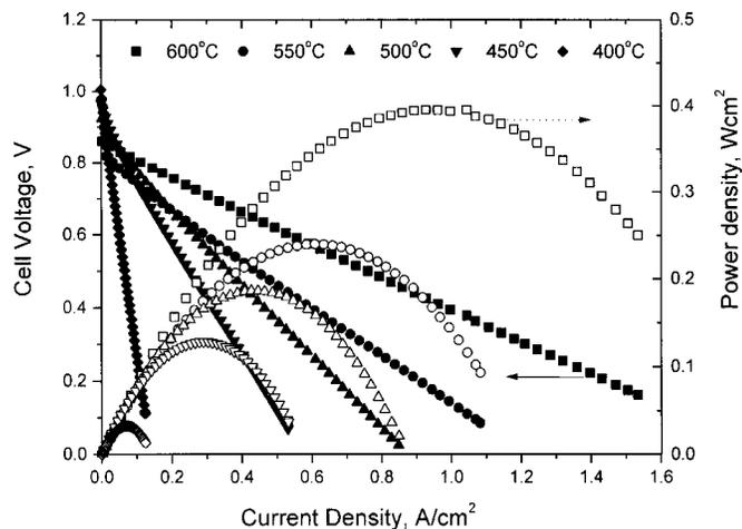
**Figure 2.** Cell voltages (solid symbols) and power densities (open symbols) as a function of current densities for an SOFC with humidified (3% H<sub>2</sub>O) hydrogen as fuel at temperatures from 400 to 600°C.
