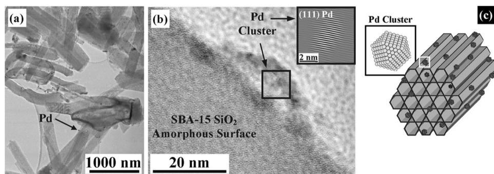
**Figure 1.** (a) General TEM view of the Pd-modified silica mesoporous material. (b) HRTEM micrograph of a Pd nanocluster placed on the mesoporous surface. The inset shows the filtered Pd (111) planes of the selected nanocluster. (c) Model proposed for the nanocluster dispersion in the Pd-modified mesoporous silica. Nanoclusters used in the model are the 561 atom Pd cuboctahedrons (with  $\sim 3$  nm lateral size).
