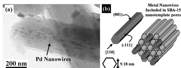
**Figure 2.** (a) 2-D bright-field TEM view of a Pd-modified SBA-15 silica mesoporous aggregate. (b) Pd-modified SBA-15 mesoporous silica model with platinum adopting nonregular hexagonal prism morphology.
