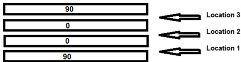
Figure 4.2. Specimen layup and planned delamination locations.
