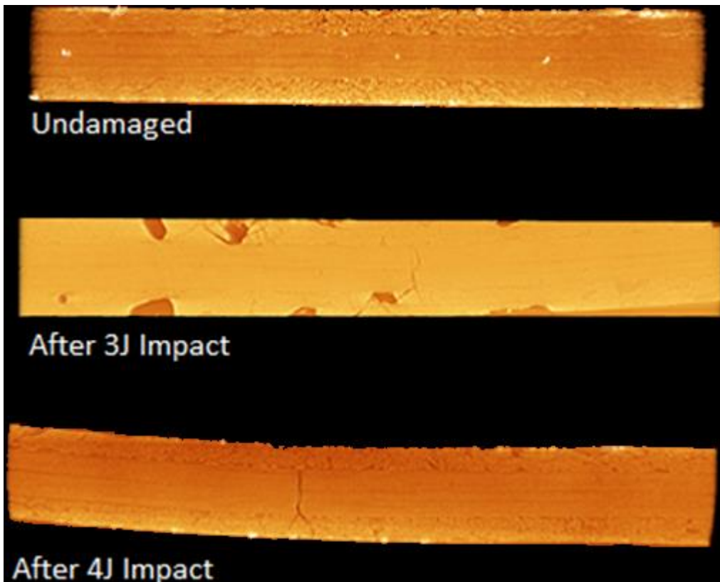
Figure 3.11. X-ray images of undamaged and damaged Cross-ply specimens.
