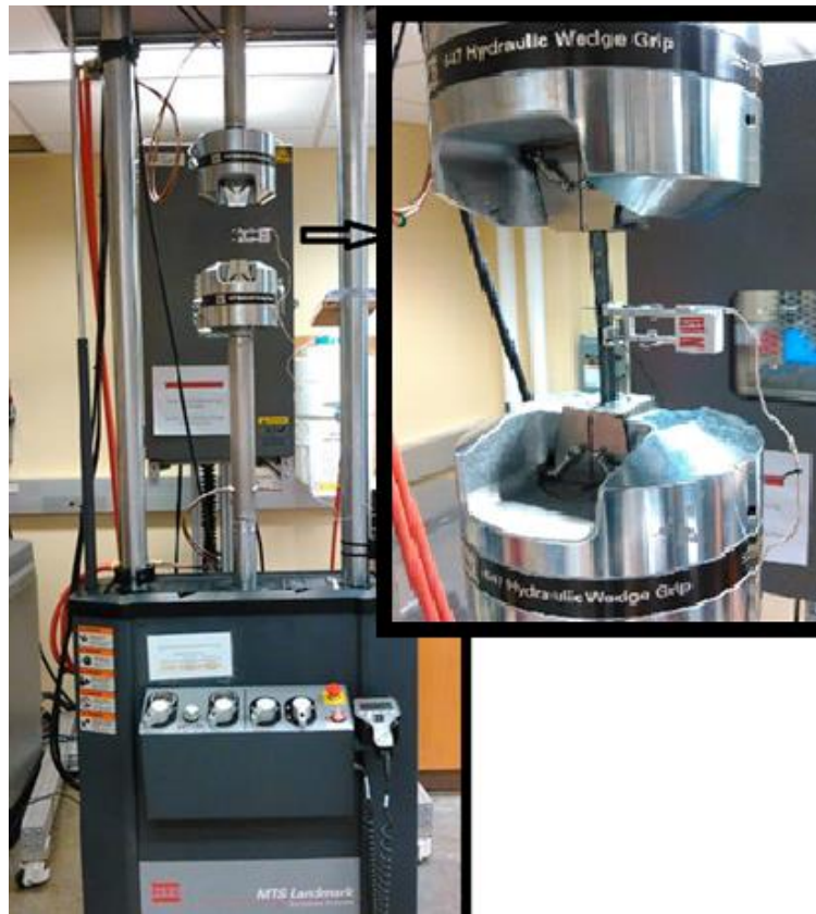
Figure 4.3. MTS machine with cross-ply specimen and extensometer
