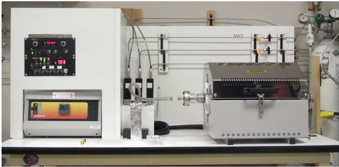
Figure 2.1 The home-build CVD graphene growth system
