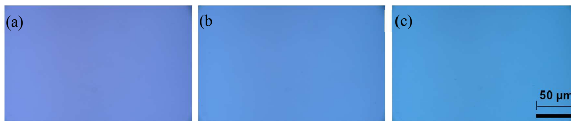
Figure 3.3 Optical Image of amorphous Boron Nitride (a) 5nm (b) 10nm and (c) 20nm grown on 300 nm SiO 2 /Si at 200 °C.
