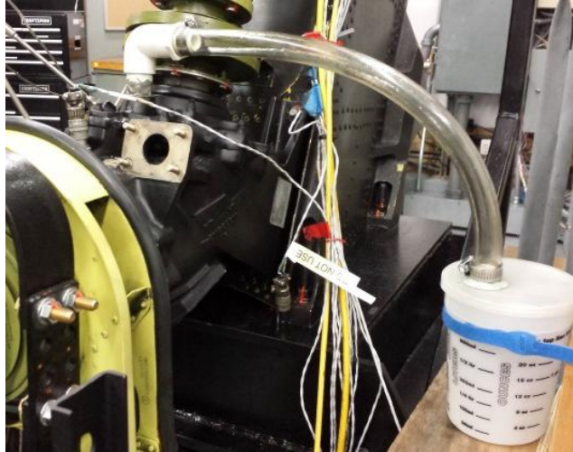
Figure 4.2 Breather port adapter setup
