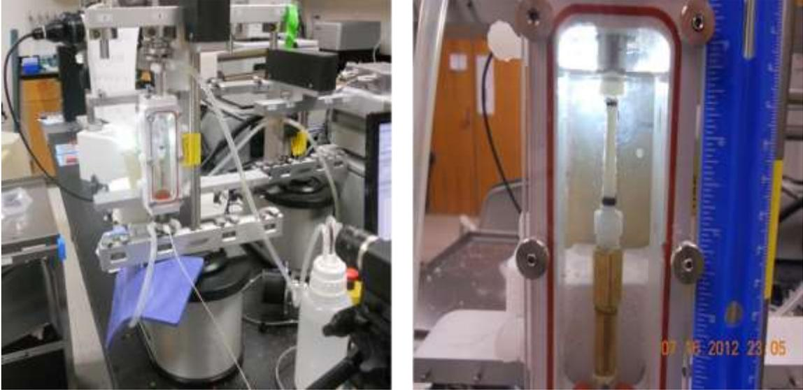
Figure 2.2. Experimental setup for extension-inflation testing of vascular specimens (Bose BioDynamic 5270).
