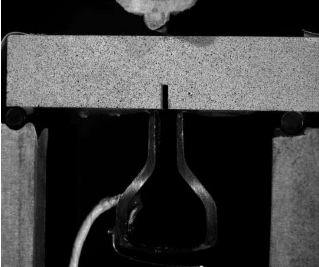
Figure 3.2 - Close-up photograph of notched beam specimen with DIC speckle pattern
