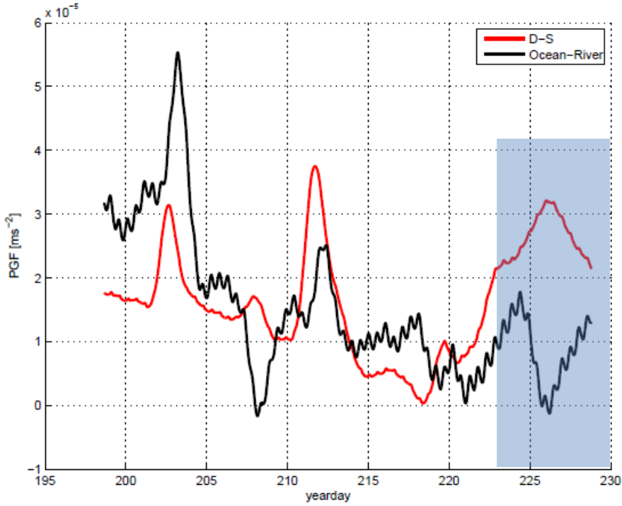
Figure 3.14 Pressure gradient force term D (red) and pressure gradient force between USGS gauging station 02171905 and USGS gauging station 02171700 (ocean-river). Blue bar shows yearday corresponding to discrepancy between both.
