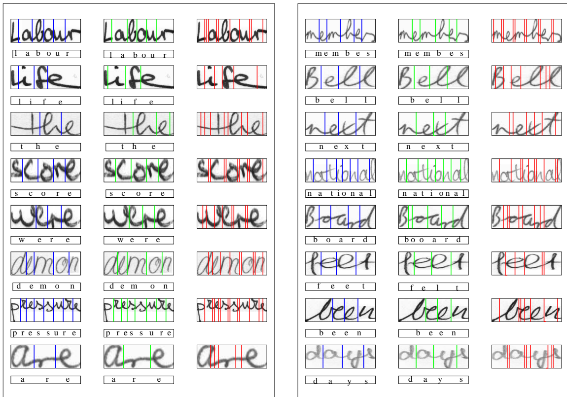
Figure 1.4: Text segmentation on a subset of the test words. For each test word, we show the segmentation from: (Left) the ground truth, (Middle) the presented method, and (Right) the dynamic programming based method [60]. The characters below the test words for the presented method (Middle column) are the recognition results from the character class corresponding to the character likeliness. The characters below the test words for ground truth (Left column) are the ground-truth characters for these words.
