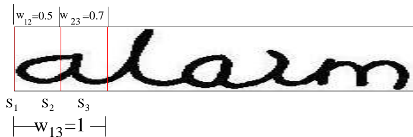
Figure 1.2: An illustration of the oversegmentation problem of dynamic programming.
