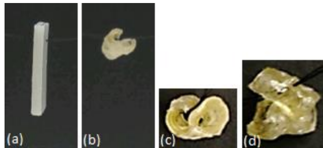
Figure 4.11 Specimen J of 1% Random Fiber Orientation Hydrogel Bilayer with fiber layer on the left (a) Before (b) After a drying period of over 12 hours (c) Side view of the hydrogel wrapping around itself (d) Front view of the specimen wrapping around itself
