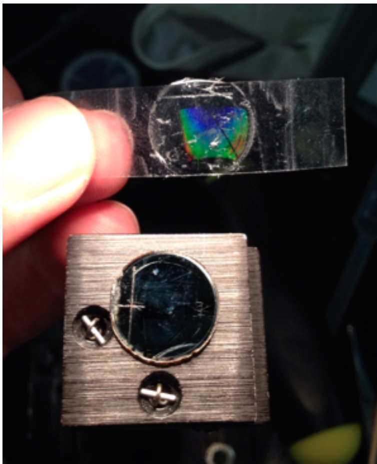
Figure 3.2 Pealed polymere film via double sided tape
