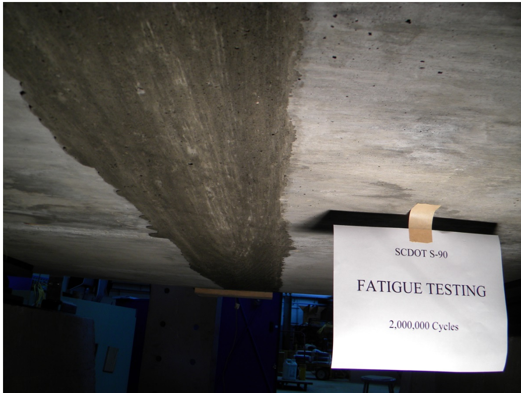
Figure 3.23: Underside of joint after fatigue loading
