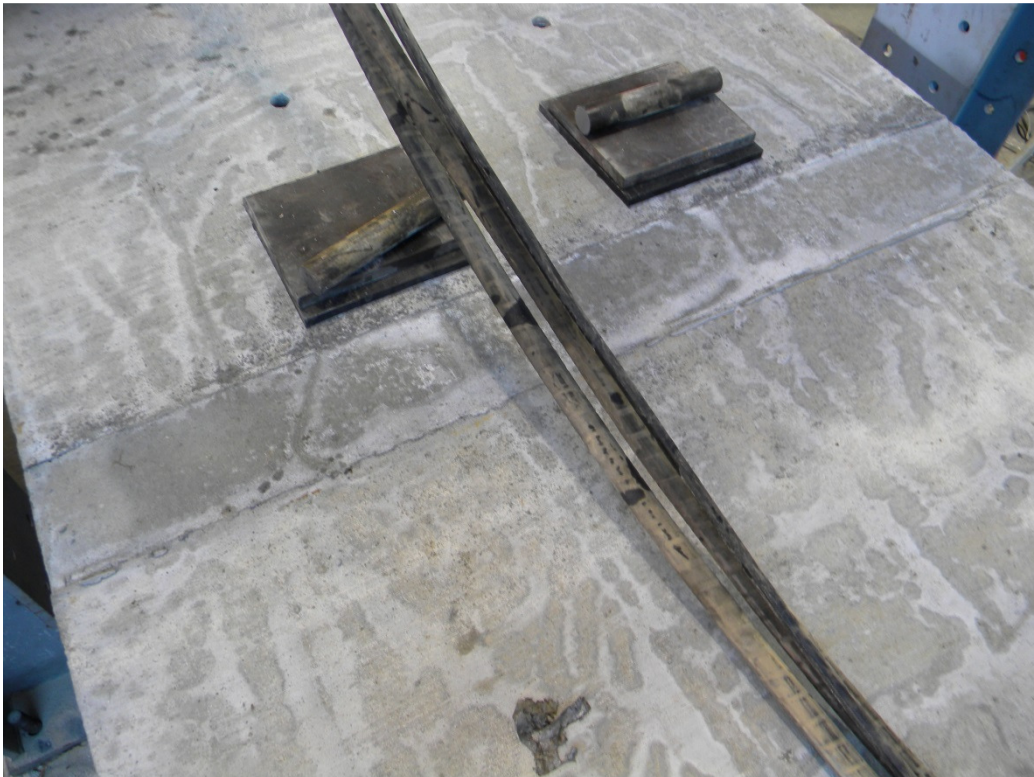
Figure 3.14: Joint following closure pour
