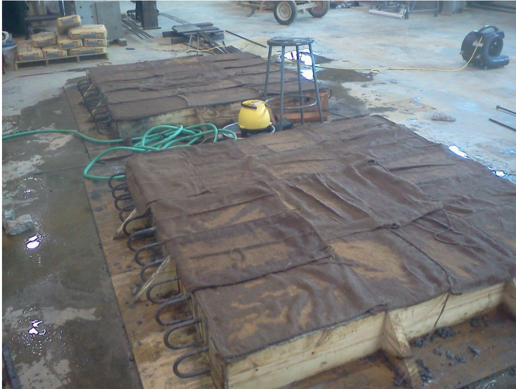
Figure 3.9: Specimens being moist cured
