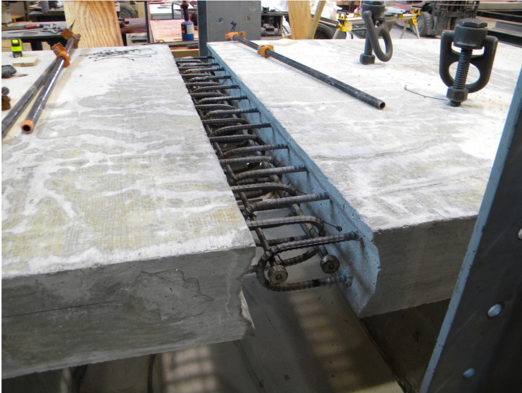
Figure 3.13: View of completed joint prior to pour
