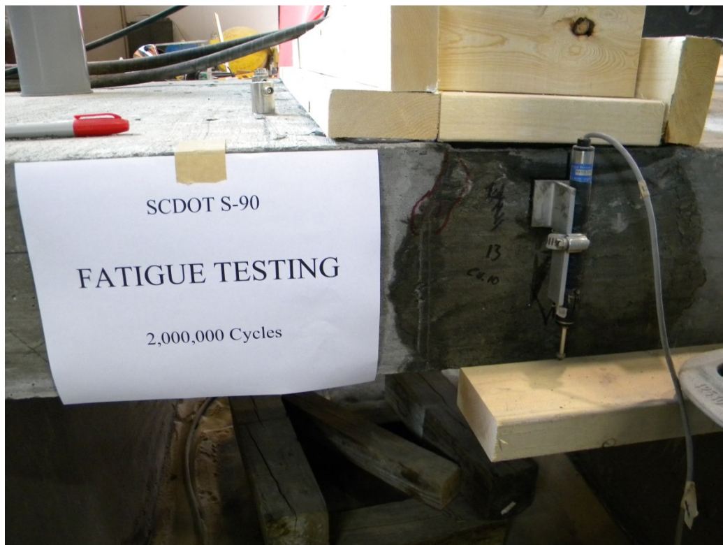
Figure 3.22: Joint condition following fatigue testing
