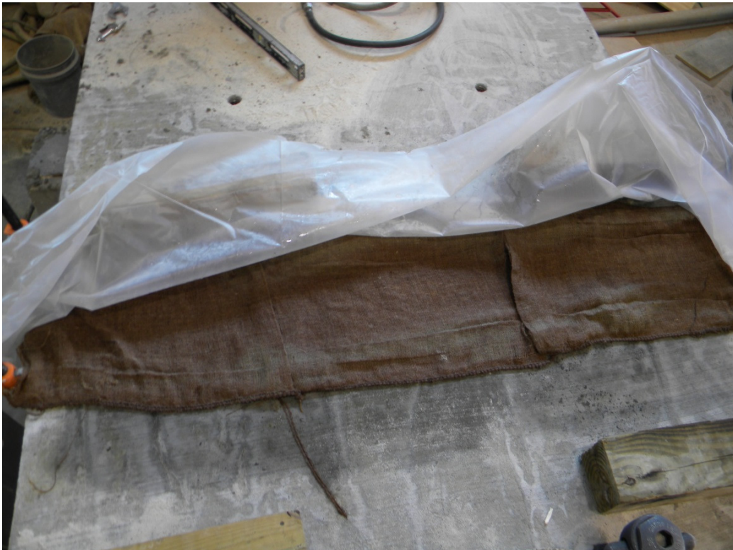
Figure 3.16: Burlap and plastic used for curing joint
