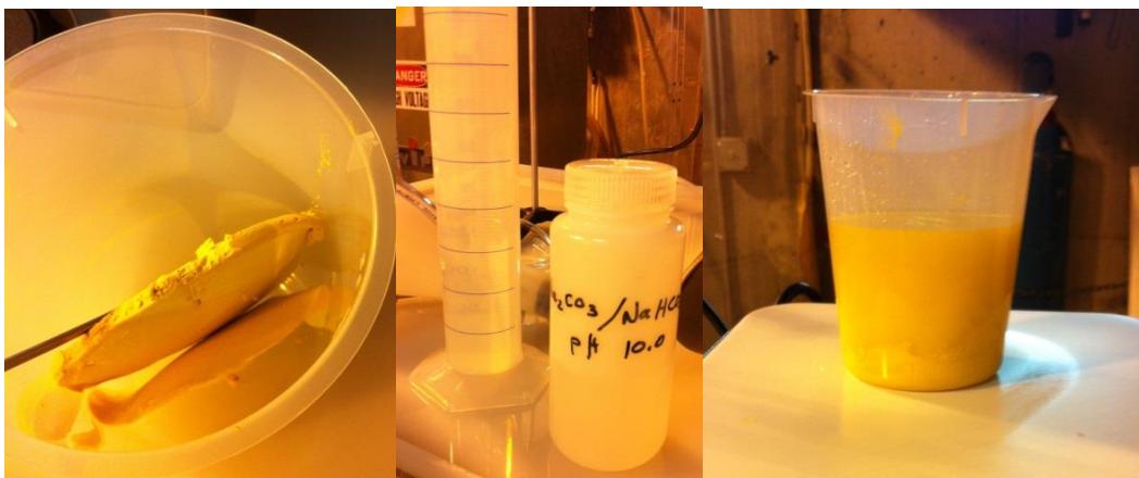
Figure 4.14 – SDU Filter Cake in Beaker, Sodium Carbonate/Bicarbonate mixture (pH=10), Slurry of SDU and 300 mL of 10% \text{Na}_2\text{CO}_3 solution
