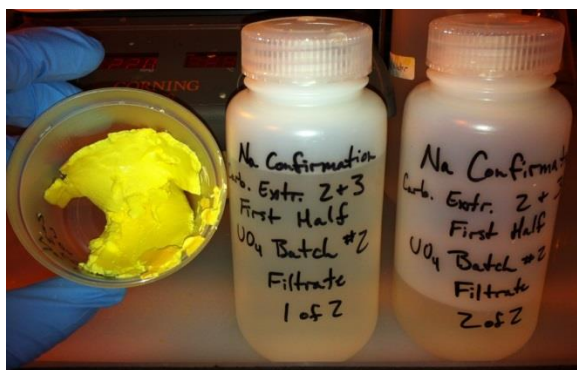
Figure 4.46 – Fifth Test Series, Batch 2, \text{UO}_4 filter cake (left) and filtrate (right).
