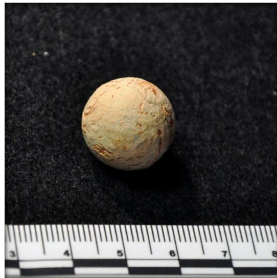
Figure 6.6 Surface dimples caused by the rolling process seen on an unfired .75 caliber musket ball
