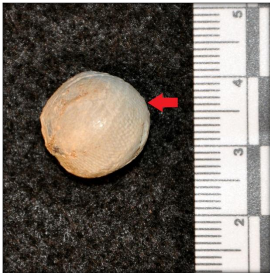
Figure 6.5 Full barrel patch mark as evidence of minimal windage in a 'smoothbore rifle'
