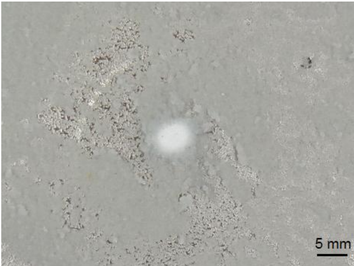
Figure 2.12 Image of the squeezed suspension of glass spheres in Dow Corning 200 Fluid 300,000 cSt with volume fraction of 0.586 showing a whiter and dryer spot at the center.
