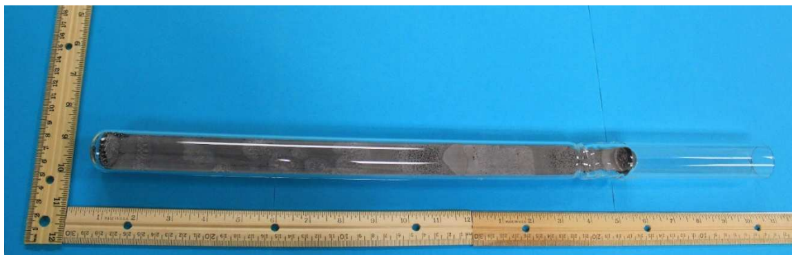
Figure 2.4. Zone refined a-Se ampoule after 27 cycles.
