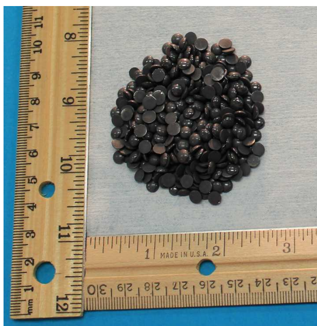
Figure 2.15. Sample #3 a-Se (As 10.2%, Cl 60 ppm) alloy pellets.
