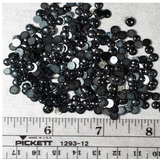
Figure 4.3. Enriched ^{10}\text{B} -doped Se (As, Cl) alloy dry pellets.
