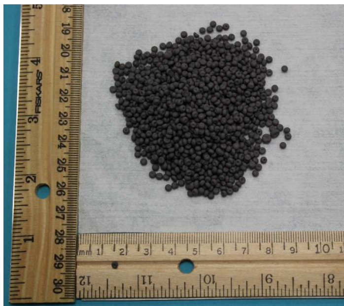
Figure 2.12. Sample#2 Se-Cl master alloy wet shots Cl-0.34%.
