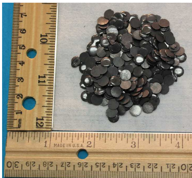
Figure 2.14. Sample #4 a-Se (As 0.52%, Cl 5 ppm) alloy pellets.
